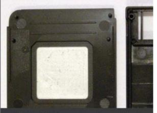
The fake iEDGE snaps together and breaks easily caused by absence of screws, normally used to secure the casing.
