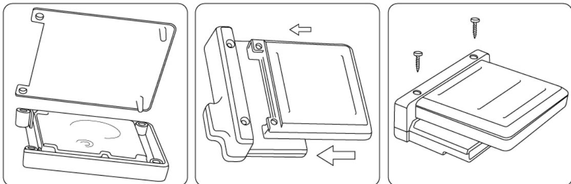
1. Remove the two screws which attach the media caddy to the rest of the media dock (if necessary) using a small cross headed screwdriver.
