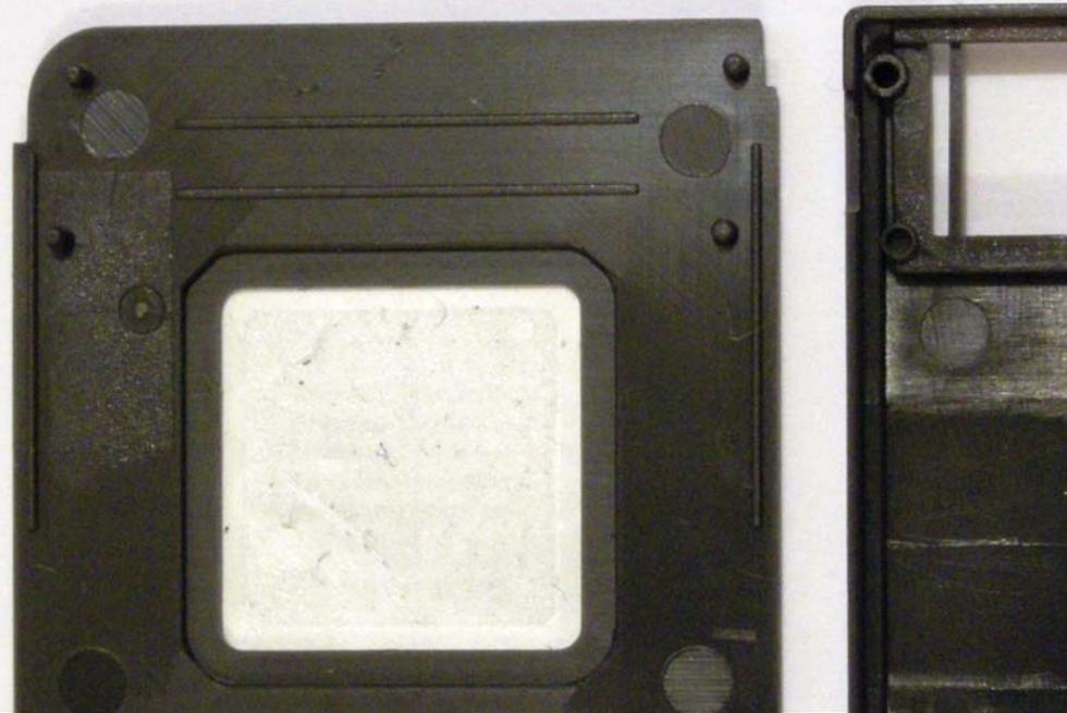
The fake iEDGE snaps together and breaks easily caused by absence of screws, normally used to secure the casing.
