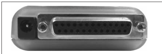
Parallel Port, Power Supply Port
