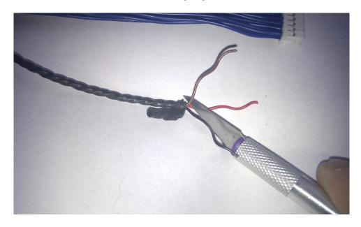
Now strip the ends of remaining 2 cables and tin them with your soldering iron, in preparation for next stage.
