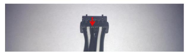
With the plug upwards (notice the pegs on top) the indicated cable is GND. The one directly below it is 3.3V.
