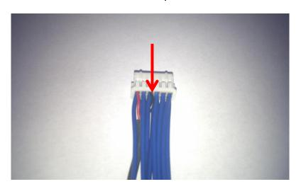
If using the CK cable – chop the small plug of the end leaving you with 3 cables
