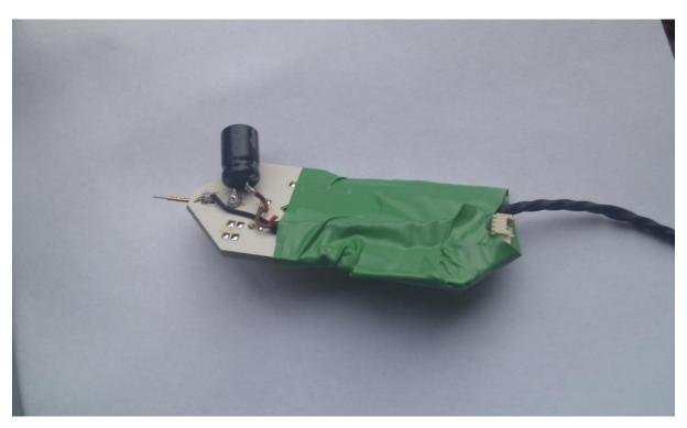
Incidentally – as I didn't want to have a charged capacitor at all time if I was using that cable for other drives – I fitted a small switch into my cable at the drive end. Cutting into the Brown wire. This is not necessary for it to work – just something I added.
