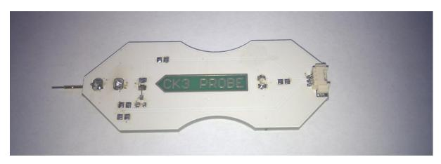
On this one, I knocked of all the surface components with my soldering iron (we are only interested in the pin itself)
