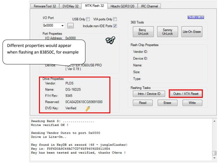
This will release a drive from **Vendor Mode** and send **ATA Reset** to the Drive. It then sends an inquiry command to the drive.
