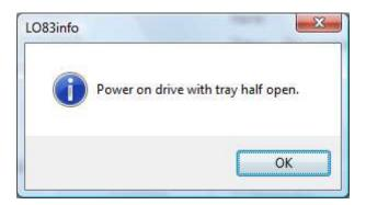
As with the original command, please ensure the drive is **fresh / power cycled as**part of setting "tray half open" , before continuing
