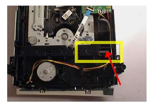
Then, pull the tray out fully and push half way back in. Now, hook it up to the PC using Connectivity Kit and SATA then power on. (If powering with Xbox – then DVD power plug must be removed before this process, with Xbox powered on – then power plug connected after tray position is set!)
