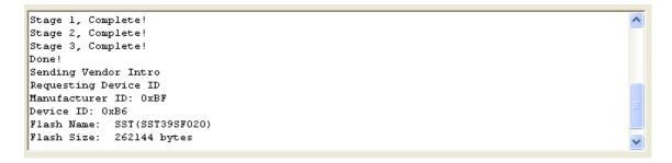
The drive should be in Vendor Mode (0x70) now and return good flash chip properties; you can check under Flash Chip Properties, Drive Properties should show "Drive in Vendor Mode!"
