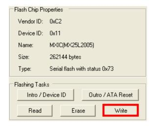
**Write** Command, will send Chip Erase prior to writing and then proceed to write the 4 banks of the firmware (banks 0/1/2/3).
