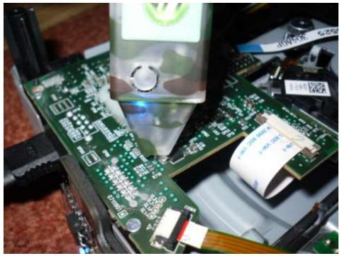
**USBXtractor Users can press the button on probe to start DVDKey32**
