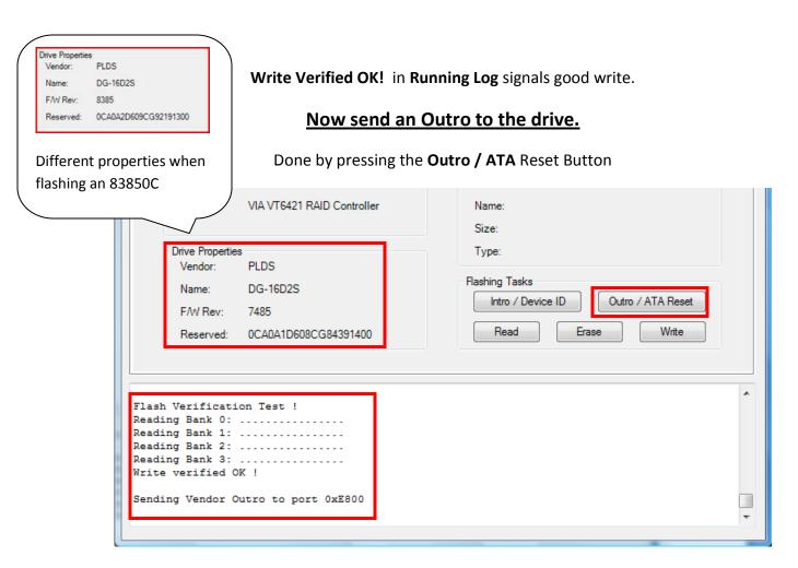
This will release a drive from **Vendor Mode** and send **ATA Reset** to the Drive. It then sends an inquiry command to the drive.
