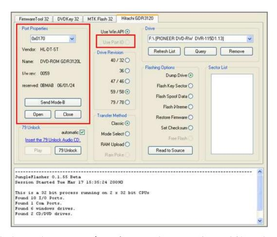
The drive needs to inquire on **I/O** port for **Raw ModeB Commands to work** (this applies to spoofed drives also)
