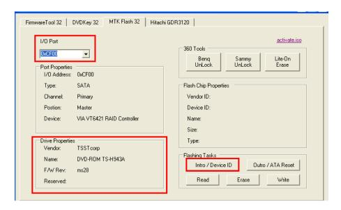
If Activate.iso worked correctly, you will get good **flash chip properties (0x70)** and drive will appear in **Vendor Mode** in **Drive Properties.**
