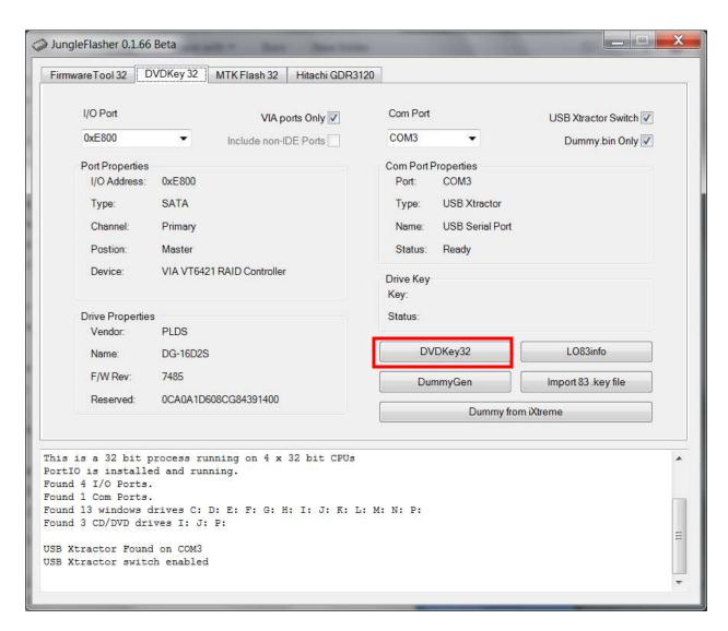
Providing serial connection was good, **DVDKey 32** will dump the key 6 times and compare each dump –
