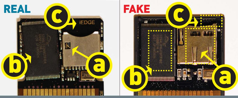
a.) The real iEDGE uses a non spring loaded Micro SD slot ensures longer life span and prevents card slot insertion failures.
